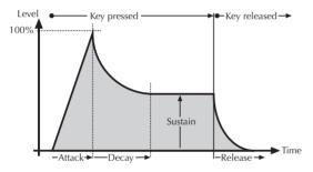
The envelope is started by pressing a key. It ascends to its maximum value at the rate determined by the **Attack** parameter. It then descends at the rate determined by the **Decay** value until it reaches the predetermined **Sustain** value. It remains at this value until the key is released. The
