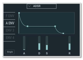
The Blofeld plug-in envelopes allow you to manipulate sound parameters via rate or timed modulations. The Blofeld offers four independent programmable envelopes for every sound program:
