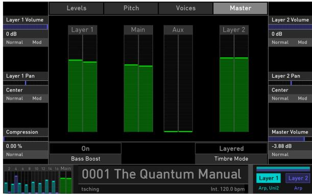
The current volume of Layer 1, 2 as well as Main and Aux volume is displayed in the gain meter representation.
