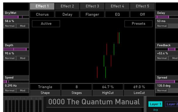
⚠ For the typical Chorus effect sound the **Dry/Wet** parameter should be set to 50%.
